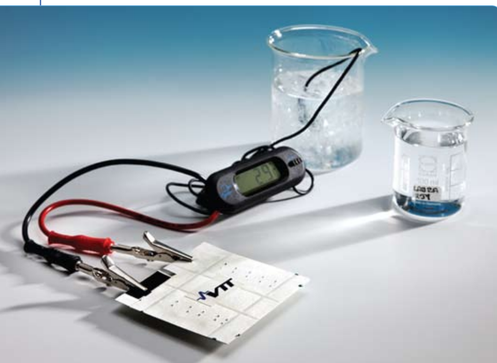
Figure 1. Demonstration of the printed biofuel cell as a power source for a digital thermometer.
