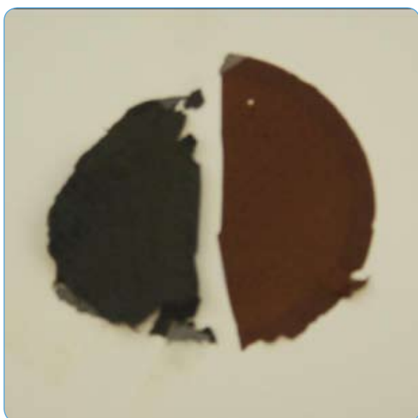
Appearance of oxidized PAN web, right, and the same sample after carbonization at 800 °C, left.
