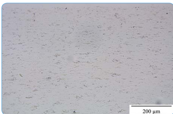
Figure 3. Optical micrograph of NFC composite made by conventional melt compounding.
