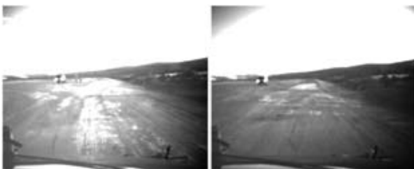
Figure 3. The captured test samples. The left-hand image was captured with a horizontal polarization filter and the right-hand image with a vertically polarized component.
