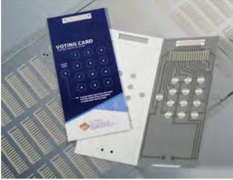
**Figure 2. Electronic voting card used at IDTechEx Printed Electronics Europe 2011.**
