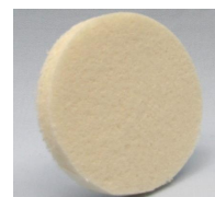
Foam formed kraft material made at VTT.
