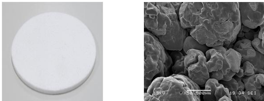
A photograph and an electron micrograph of a 100 mm sample of a sintered UHMWPE absorption material developed at VTT.
