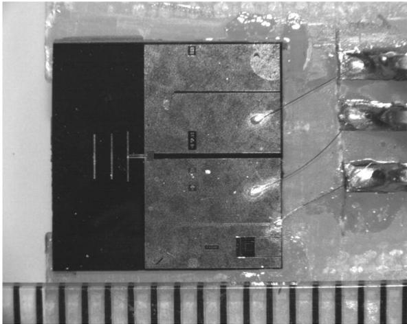
Fig. 9. Transponder used in measurements: on the left is the antenna. The Schottky diode is placed at the feed of the antenna, on the right side of which there is a low-pass filter. On the right, the baseband connector is seen. On the scale below, one tick is 1 mm.
