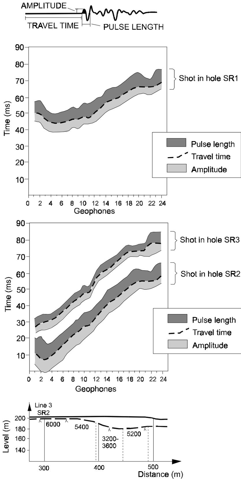
Figure 7a. Attenuation of amplitudes along the survey line from several rifle gun shots to water-filled boreholes in Kuhmo (based on Okko 1991b).
