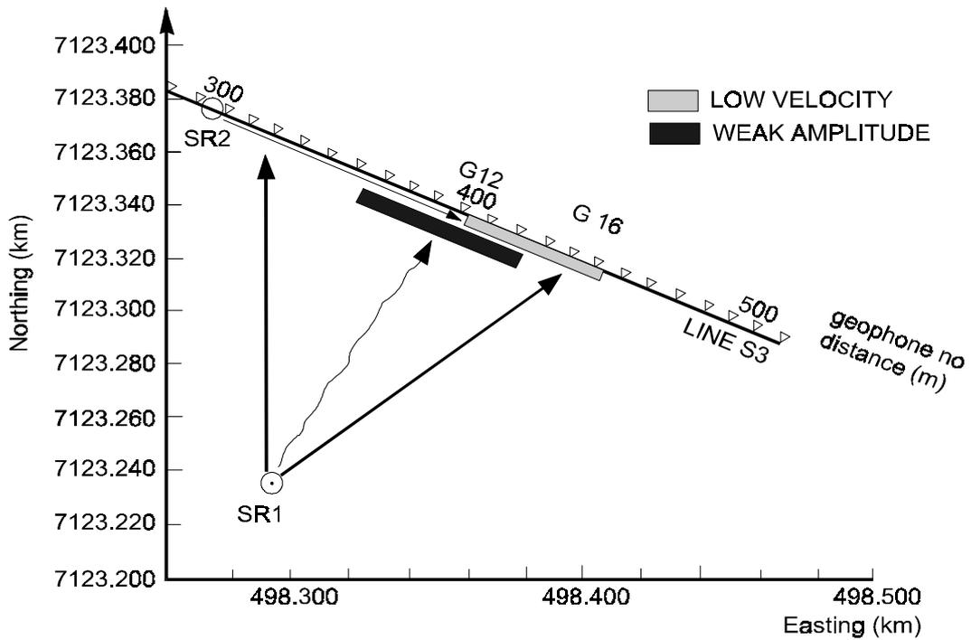
Figure 7b. The interpretation of the attenuation of amplitudes and decrease of seismic velocity from several rifle gun shots to water-filled boreholes in Kuhmo (Okko 1991b).
