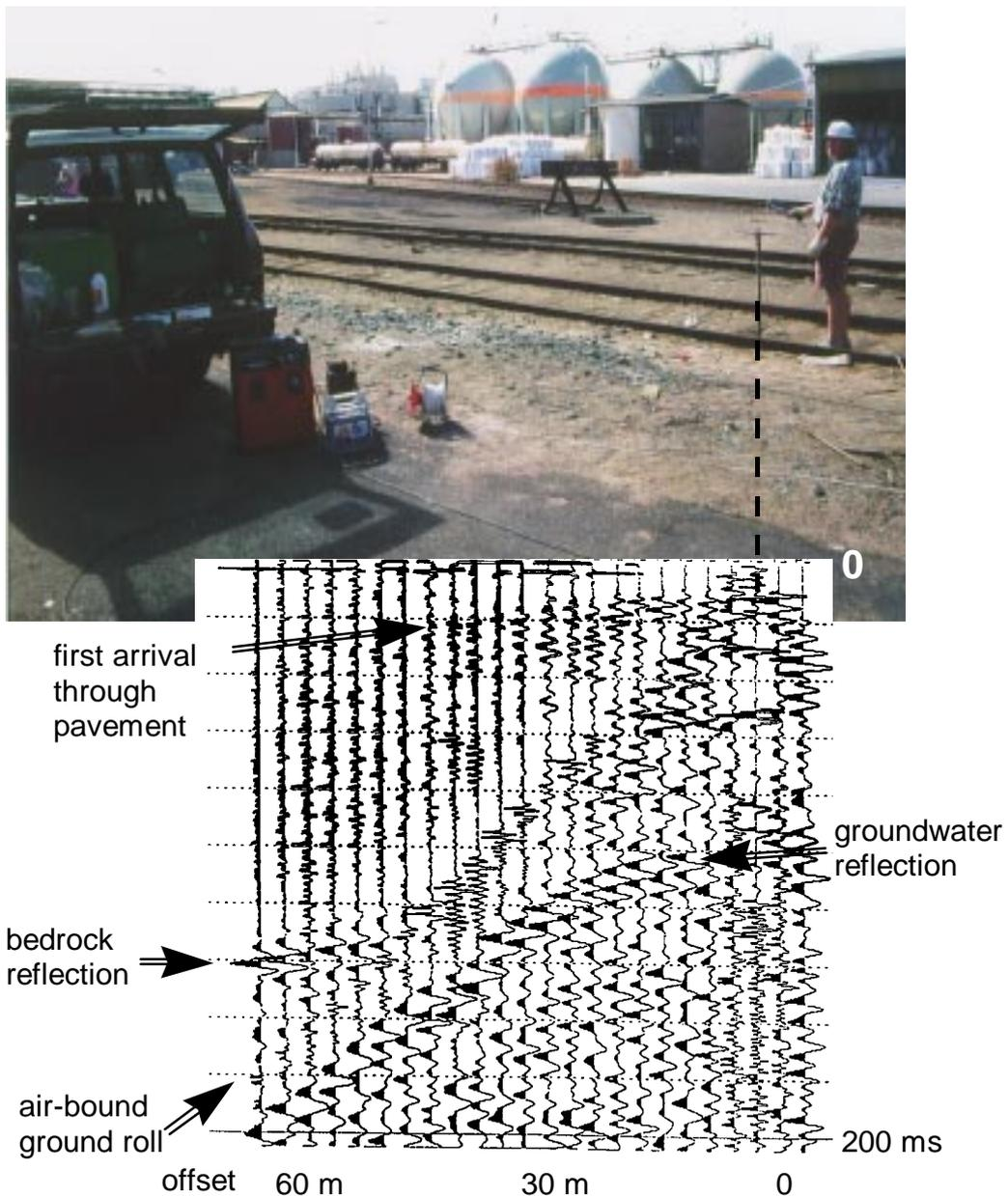
*Figure 5. High-frequency seismic record with reflections from groundwater and bedrock in the industrial area at Harjavalta. In order to avoid additional noise due to poor seismic contact with the ground, the buffalo gun and the single geophones were located on as undisturbed ground as possible. The geophone spacing was squeezed to 3 m to improve coherency.*
