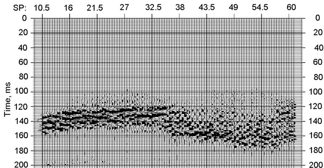
*Figure 6. Processed reflection seismic 6-fold CDP stack focused on the visualization of the bedrock topography at 120 - 160 ms: the 55 m wide bedrock depression is located between CDP stations 39 and 57.*
