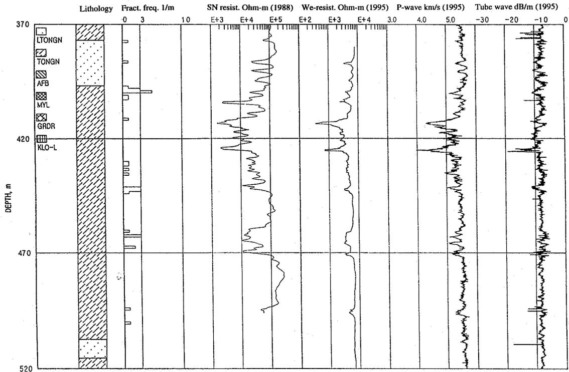
Figure 8. Geophysical logs in hole RO-KR2 Kuhmo before and after grouting of the major fracture zone at interval 410 - 430 m. The attenuation of tube waves reveals the unsuccessful grouting at 423 - 425 m (Okko 1996).
