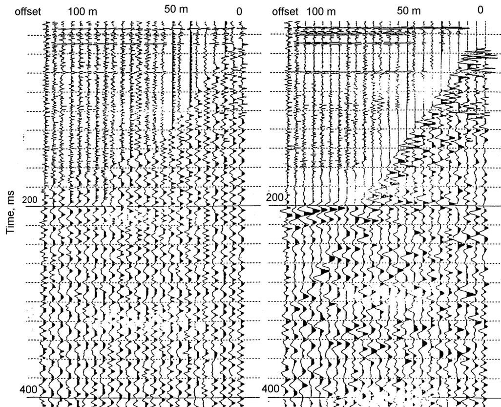
*Figure 4. High-frequency seismic record from a dynamite source at Harjavalta recorded with 5 m channel spacing and displayed with two AGC windows: on the left the 6 ms window is short and the refracted arrivals are visible, on the right the window is 80 ms long and the bedrock reflection is clear on the far channels.*
