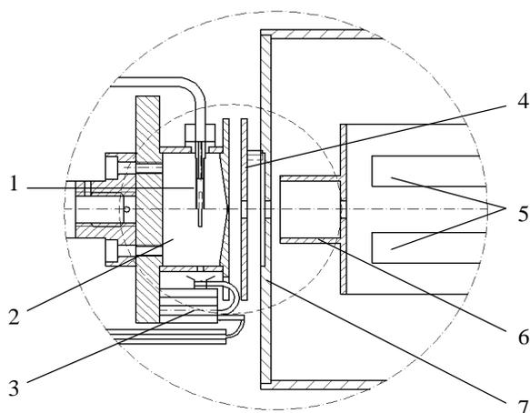
Figure 6.6. Enlarged figure of the inlet/ion source of the DCI-MIMS system. **1** Membrane, **2** ion volume, **3** filament, **4** extractor lens, **5** field (quadrupole analyzer), **6** focus lens, **7** grounded plate (divider of the vacuum chamber).
