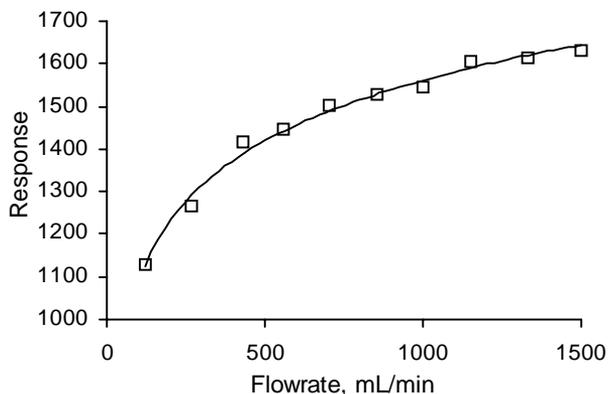
Figure 5.1. The response of toluene ( $m/z$  91) as a function of the flow rate of the sample gas. The concentration of toluene was about  $3.3 \text{ mg/m}^3$ , and the thickness of the sheet membrane was  $100 \text{ }\mu\text{m}$ .
