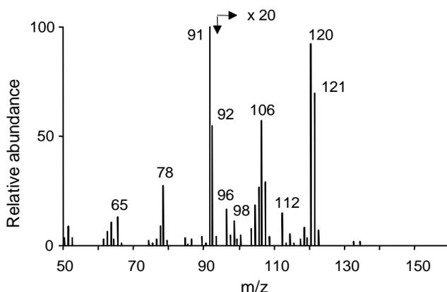
*Figure 4.1. Background subtracted mass spectrum of a contaminated groundwater sample, W04, measured on-site with MIMS. Note that the ion intensities are multiplied by a factor of 20 after the ion  $m/z$  93.*
