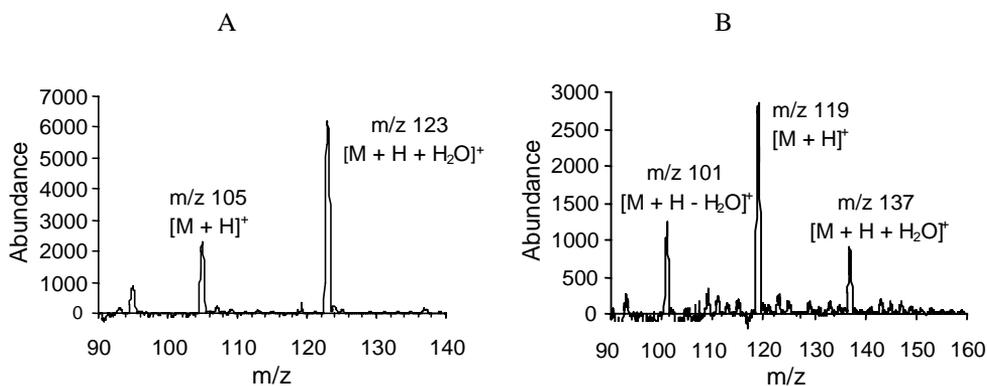
Figure 6.8. Water CI mass spectra of (A) malonic acid and (B) succinic acid. The mass spectra are background subtracted, and the concentrations of analytes are about 1 g/L.
