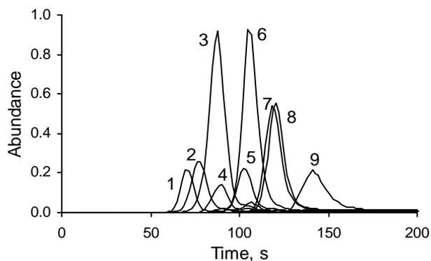
Figure 5.5. TPD-MIMS desorption profiles of a gas sample (25 mL) containing a mixture of the following compounds: **1** *trans*-1,2-dichloroethene, **2** chloroform, **3** carbon tetrachloride, **4** trichloroethene, **5** toluene, **6** tetrachloroethene, **7** xylenes, **8** styrene and **9** 1,2-dibromo-1,2-dichloroethene.
