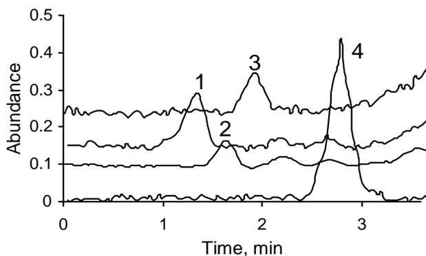
Figure 5.8. TPD-MIMS data of a gas sample (25 mL) containing the following compounds in low concentrations: **1** dichloromethane 6.0 ng ( $m/z$  84), **2** *trans*-1,2-dichloroethene 7.8 ng ( $m/z$  61), **3** chloroform 5.5 ng ( $m/z$  83) and **4** tetrachloroethene 3.6 ng ( $m/z$  166) using HayeSepD adsorbent.
