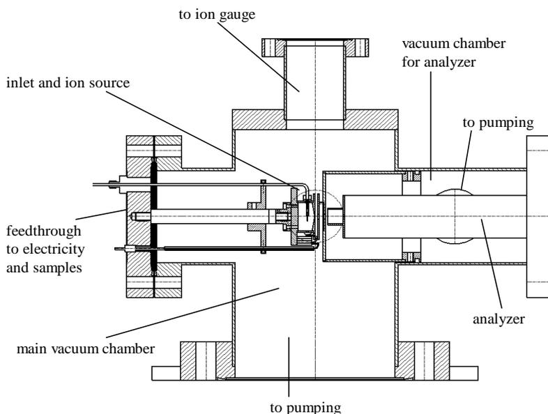
Figure 6.5. Vacuum chambers, membrane inlet, ion source and ion optics of the DCI-MIMS system.
