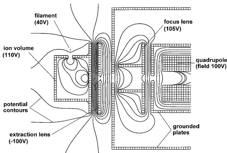
Figure 6.4. SIMION ion optics simulation of a new inlet/ CI source design.
