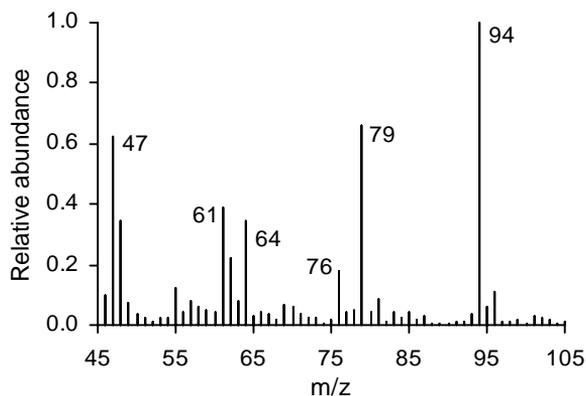
Figure 5.4. Mass spectrum of an air sample in a gas bag spiked with  $374 \mu\text{g}/\text{m}^3$  of dimethyl sulfide,  $371 \mu\text{g}/\text{m}^3$  of dimethyl disulfide and  $178 \mu\text{g}/\text{m}^3$  of ethylmethyl sulfide.
