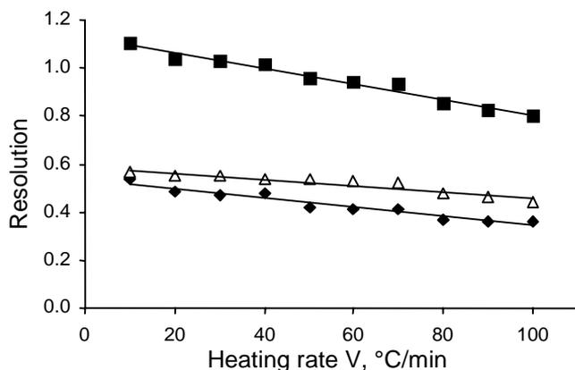
Figure 5.7. Resolution of chloroform, trichloroethene and toluene on Tenax TA as a function of heating rate ( $^{\circ}\text{C}/\text{min}$ ). ■ Resolution of chloroform and toluene,  $\Delta$  resolution of trichloroethene and toluene and  $\blacklozenge$  resolution of chloroform and toluene. The helium flow rate for purging was  $50 \text{ mL}/\text{min}$ .
