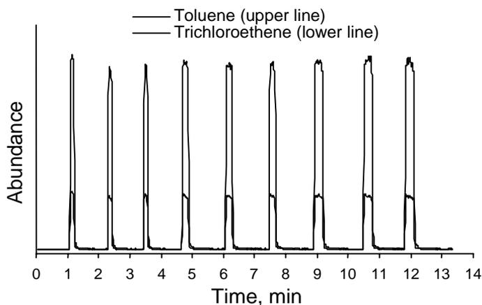
*Figure 5.3. Three successive samplings of toluene ( $m/z$  91) and trichloroethene ( $m/z$  130) were made with three different sampling times of 5, 10 and 15 seconds. The thickness of the membrane was  $25 \mu\text{m}$  and the concentrations of toluene and trichloroethene were  $700 \mu\text{g}/\text{m}^3$ .*
