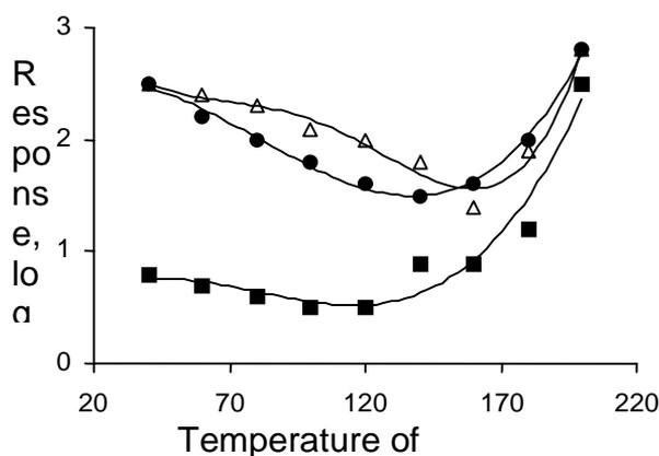
Figure 5.2. The responses of toluene ( $\Delta$ ,  $m/z$  91), trichloroethene ( $\bullet$ ,  $m/z$  130) and background ( $\blacksquare$ ,  $m/z$  200) as a function of the temperature of the membrane inlet. The concentrations of the compounds were about  $3.3 \text{ mg/m}^3$  and the thickness of the membrane was  $100 \text{ }\mu\text{m}$ .
