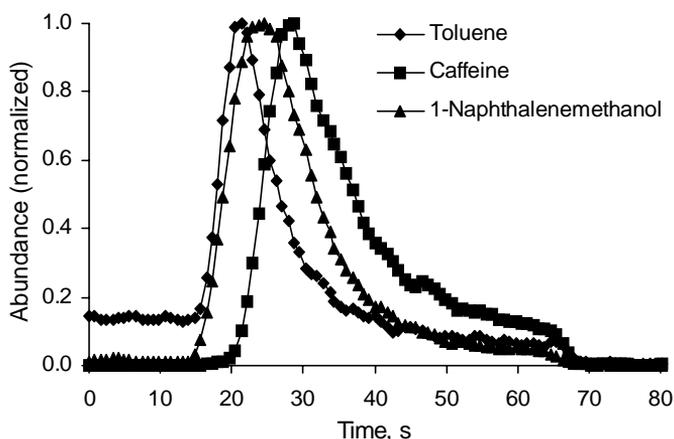
Figure 6.1. T&R-MIMS desorption profiles of toluene ( $m/z$  91 monitored), 1-naphthalene methanol ( $m/z$  158 monitored) and caffeine ( $m/z$  194 monitored) obtained during the passage of a 50-second airplug.
