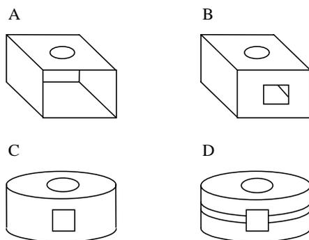
*Figure 6.3. The configurations of the ion volume studied with the SIMION ion optical program.*
