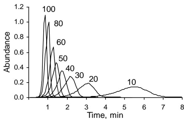
Figure 5.6. Desorption profile of toluene from Tenax TA at different heating rates ( $^{\circ}\text{C}/\text{min}$ ).
