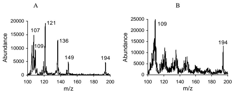
*Figure 6.2. T&R-MIMS mass spectra of a typical cup of (a) tea and (b) coffee. The spectra represent the average of 6 successive scans obtained during the release period.*
