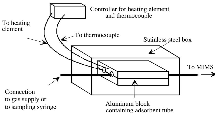
Figure 2.1. Schematic diagram of the TPD-MIMS system.
