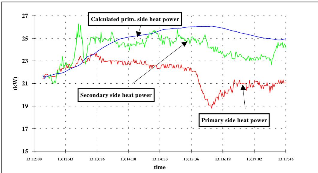
Figure 22. The primary and secondary side heat powers calculated from a heat exchanger's measured operating values as well as the primary side heat power
