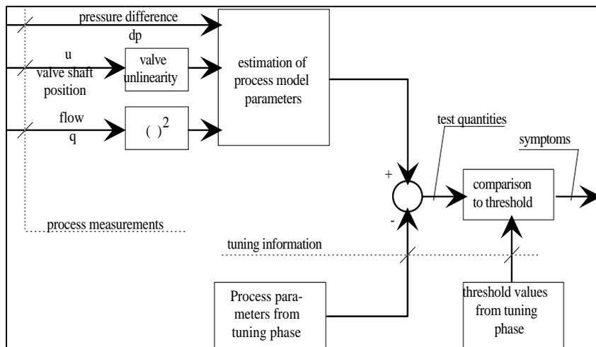
Figure 8. Block diagram of the parameter error method.
