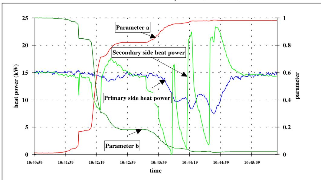
Figure 18. Tuning of parameters *a* and *b* of the dynamic calculation model according to the method as well as the heat powers of the primary and secondary side which were used as tuning data. The heat powers have been calculated from measured values. The values of the parameters at the end of the tuning are  $a =$
