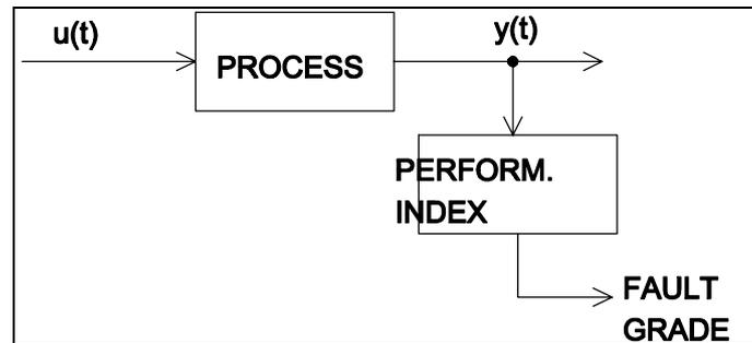
*Figure 2. Performance monitoring and classification of a process output as an independent operation.*
