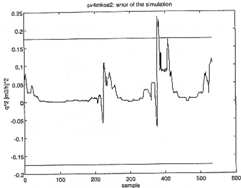
Figure 15. Residual of simulation of  $q^2$ . The residual is the difference between measured process value and respective simulated one.
