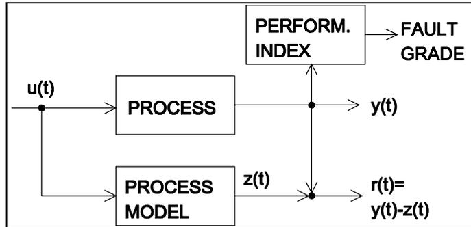
Figure 3. Parallel operation of a performance classifier and model-based fault detection.
