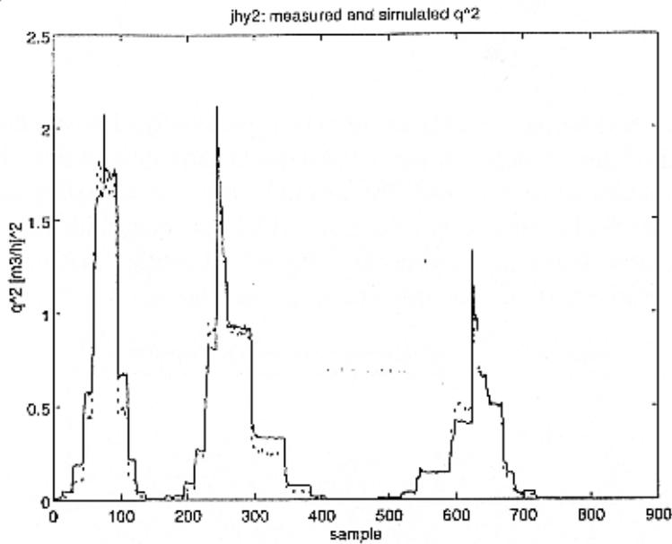
Figure 12. Simulation of  $q^2$ . Simulation done with tuning data.
