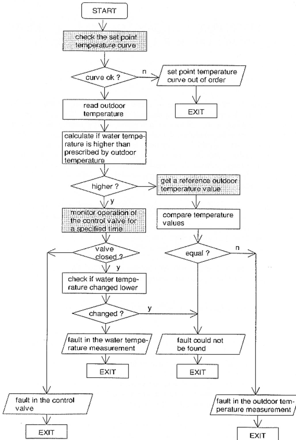
Figure 25. A flowchart of the fault localization procedure. The procedure finds a fault when the symptom is high heating water temperature. Darkened boxes refers to actions taken by the user.
