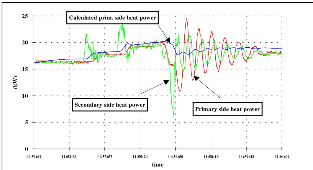
Figure 20. The heat powers of the primary and secondary side calculated from the heat exchanger's measured operating values. The figure also shows the primary side's heat power calculated with the model according to the power balance
