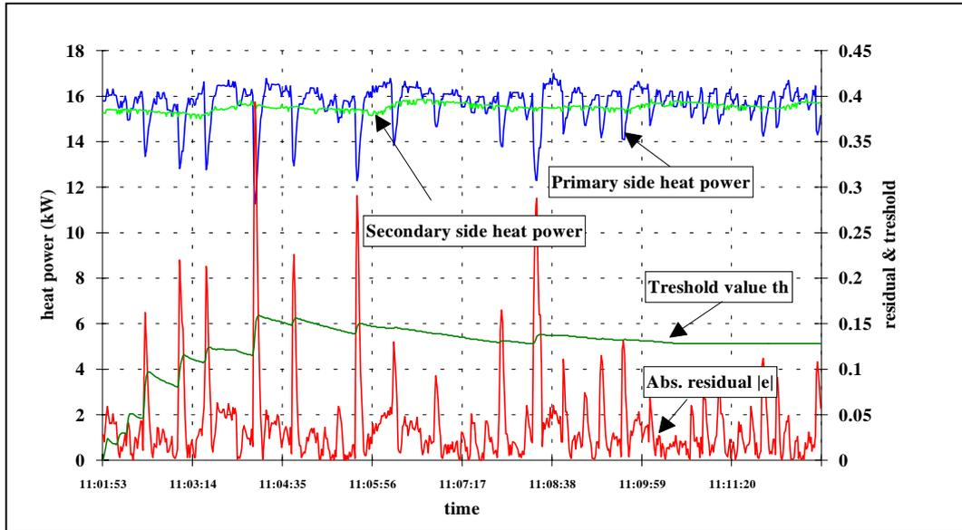
Figure 19. Tuning of the threshold according to the method. The tuning data used are the residual, which is the relative error of the primary side's heat power determined from the measured values and calculated with the dynamic model. A value of 0,128 (95% reliability limit) was obtained as the threshold.
