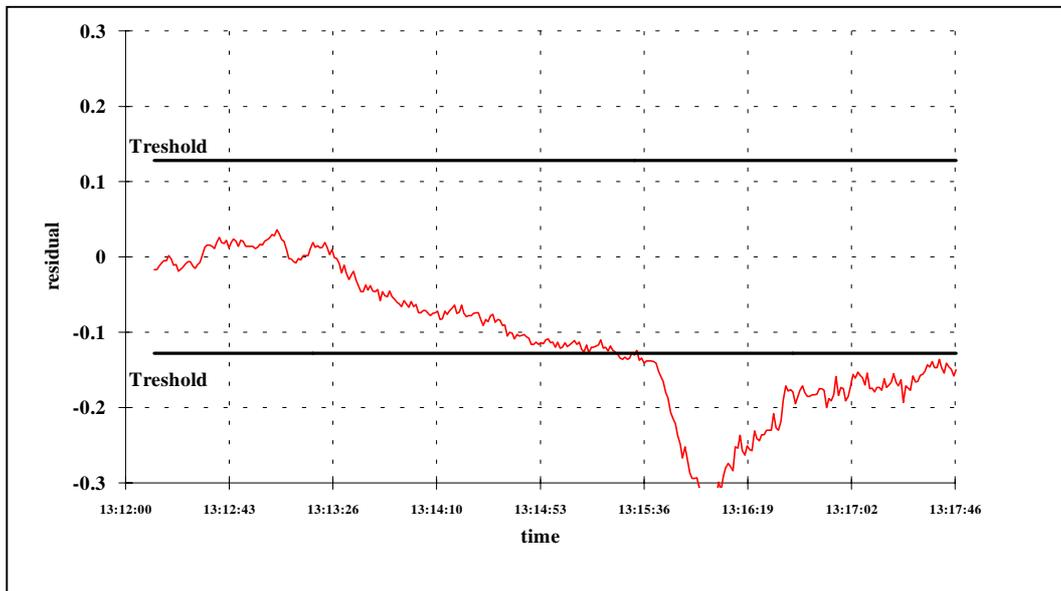
Figure 23. The relative error  $e$  of a heat exchanger's measured and calculated primary side heat power with the load period according to Figure 22.
