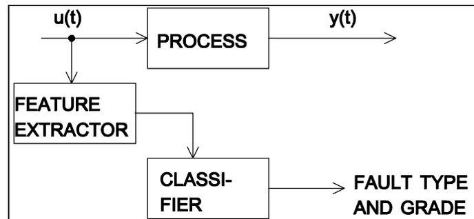
*Figure 5. Fault detection and classification of a pattern recognition system with embedded performance indices.*
