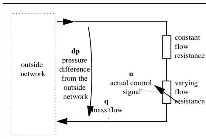
Figure 6. Electrical circuit analogy of the flow route and control valve.
