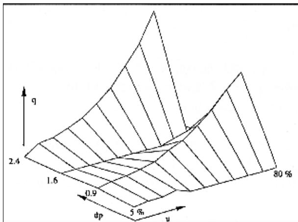
Figure 10. Process characteristic curves of figure 8 plotted as a surface (mesh-plot). The flow value remains in zero at  $dp$  value 1.6 because there has not been any measurements at that value. In reality the value of  $q$  increases continuously with value of  $dp$ .
