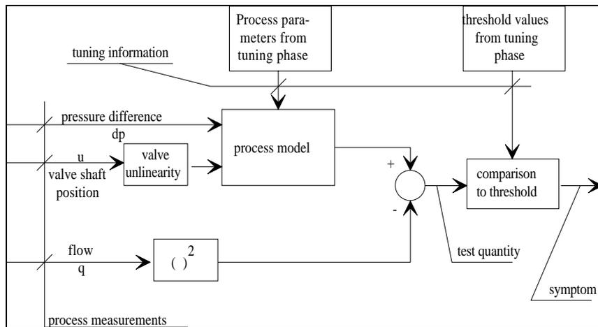
Figure 7. Block diagram of the output error method.
