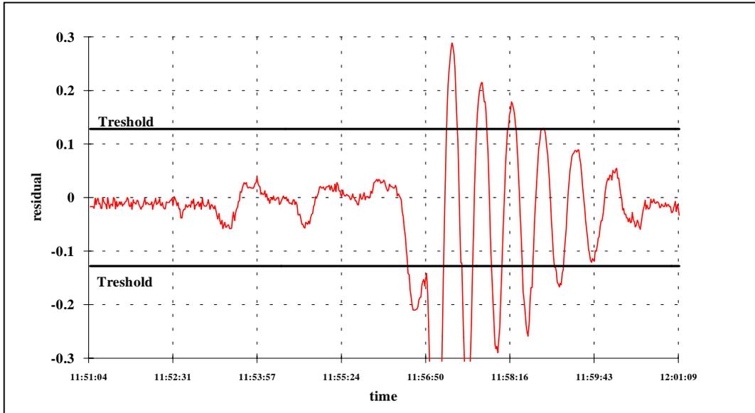
Figure 21. The relative error  $e$  of a heat exchanger's measured and calculated primary side heat power with the load period according to Figure 20.
