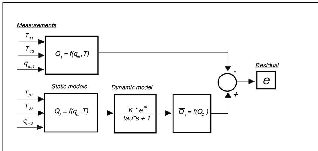
Figure 16. The calculation model of the heat power balance method. Subindex 1 corresponds to the heat exchanger's primary side, and 2 to the secondary side.
