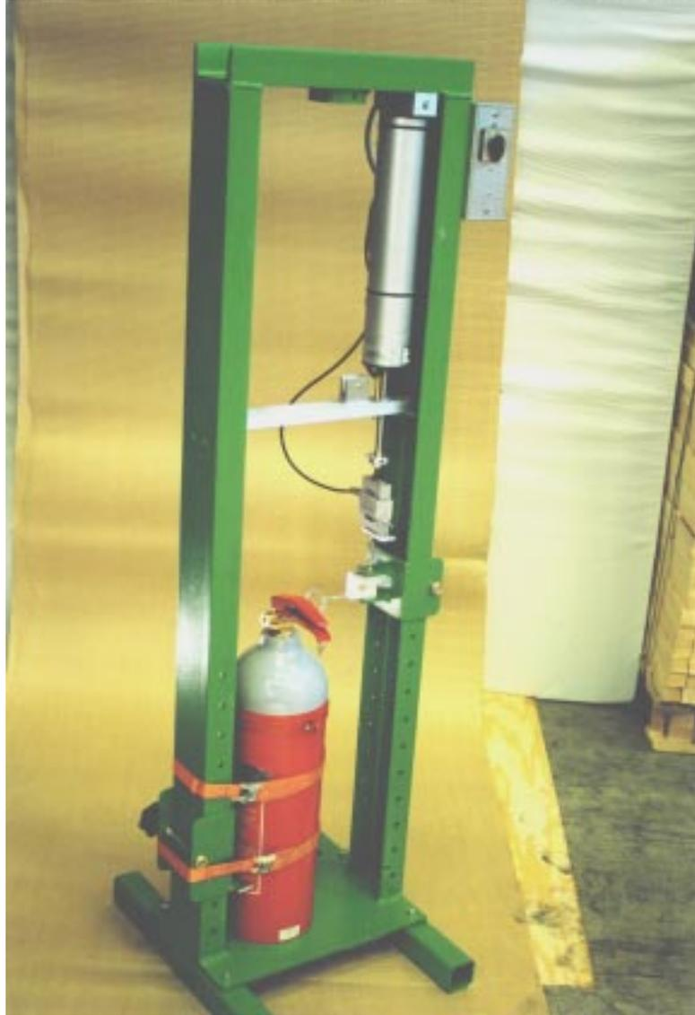
*Figure 2. Testing the safety device of a CO<sub>2</sub> extinguisher – general view.*
