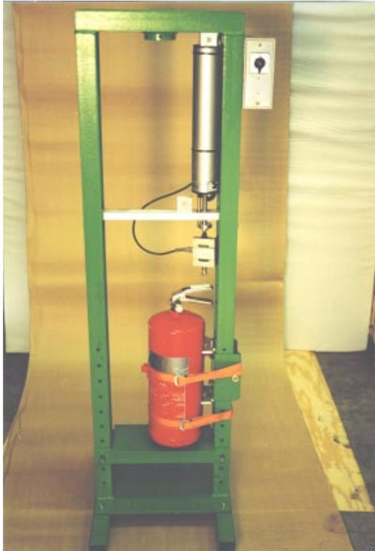
*Figure 1. General view of the test equipment used for measuring the forces required to activate a portable fire extinguisher and to release the safety device of the extinguisher. The photograph shows the new version of the equipment which was developed in this study. It is a redesigned version of the original equipment from 1987 [4].*
