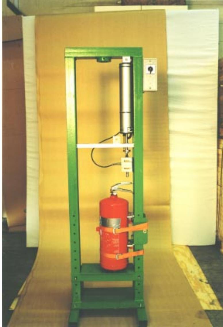
*Figure 4. Testing the actuating device of a foam extinguisher – general view.*
