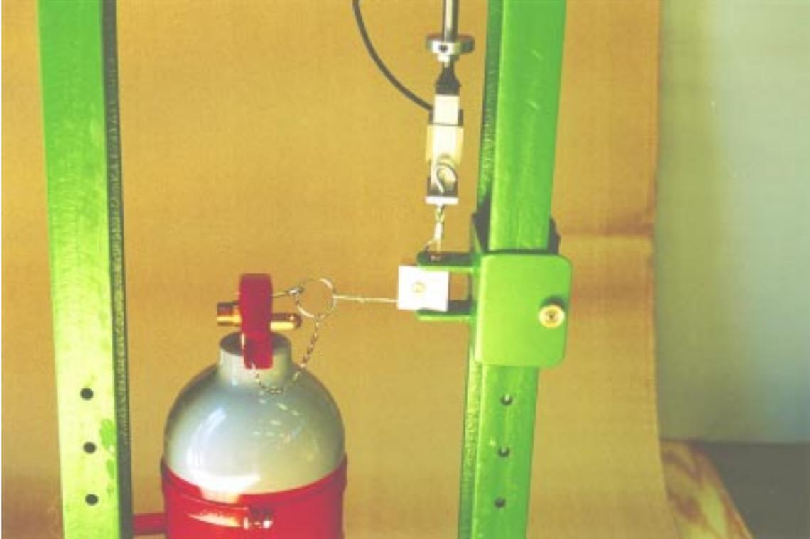
*Figure 3. Testing the safety device of a CO<sub>2</sub> extinguisher – detailed view.*
