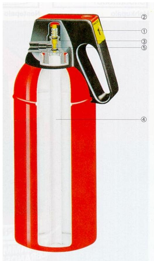
*Figure 1. A stored pressure portable fire extinguisher with a finger trigger operating device. No. 1 is the safety device, No. 2 the finger trigger device, No. 3 the control valve, No. 4 the diptube and No. 5 the nozzle [1].*
