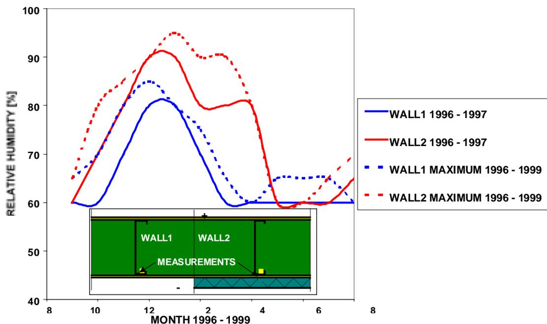
Figure 10. Monthly maximum of relative humidity in the external walls of the Ylöjärvi steel buildings. Measurements on the outer flange of the steel members.
