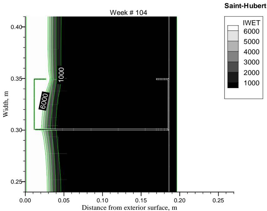
Figure 15. Contour plot of the accumulated time of wetness in the layers of the steel frame wall without exterior insulation. Exterior conditions: Saint Hubert weather data. Length of the simulated period is 2 years (104 weeks) /14/.
