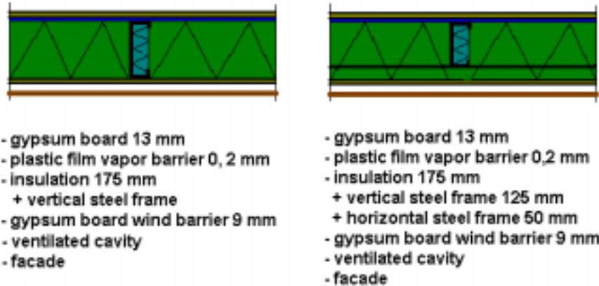
Figure 1. Single and double framed wall structures used as exterior wall in Finland.
