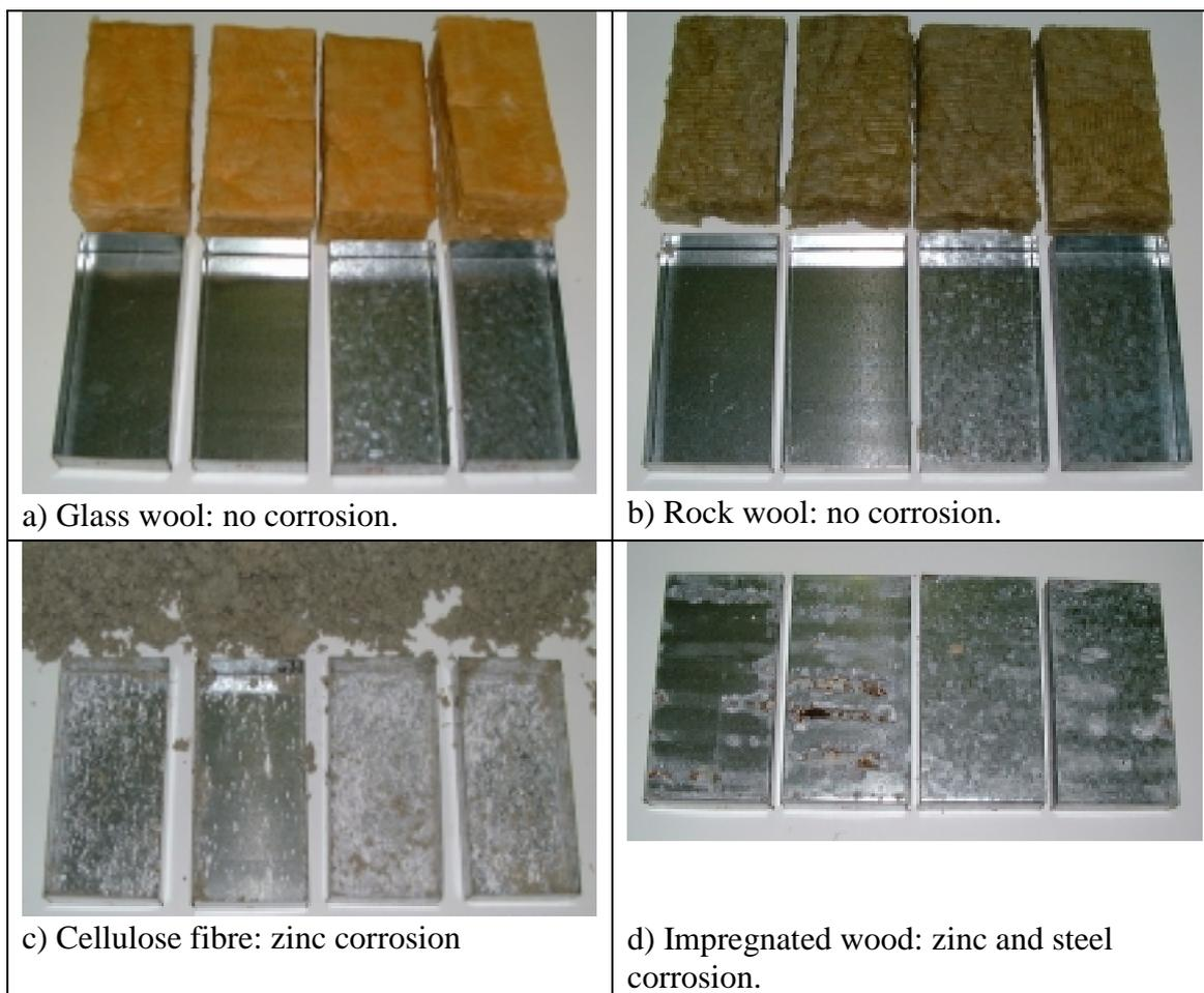
*Figure 12. Long-term corrosion test with steel members in contact with other materials. Test conditions +23°C and 85% relative humidity. Test time 35 000 hours.*
