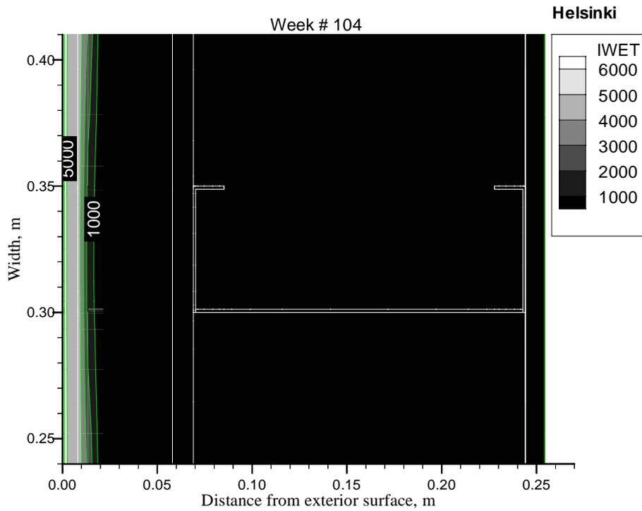
Figure 16. Contour plot of the accumulated time of wetness in the layers of the steel frame wall with 50-mm exterior insulation. Exterior conditions: Helsinki weather data. Length of the simulated period is 2 years (104 weeks) /14/.
