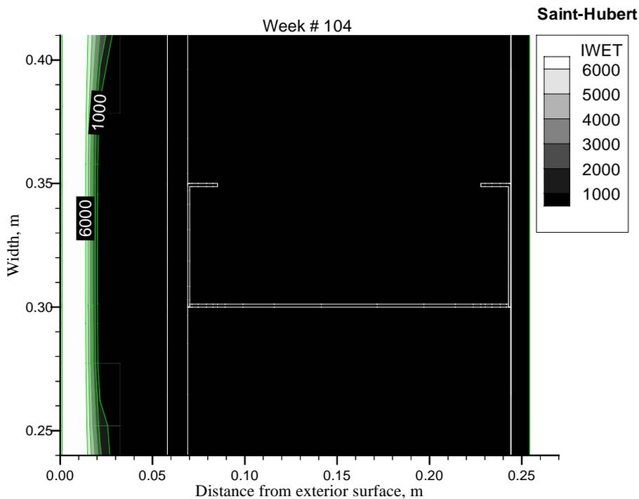
Figure 17. Contour plot of the accumulated time of wetness in the layers of the steel frame wall with 50 mm exterior insulation. Exterior conditions: Saint Hubert weather data. Length of the simulated period is 2 years (104 weeks) /14/.
