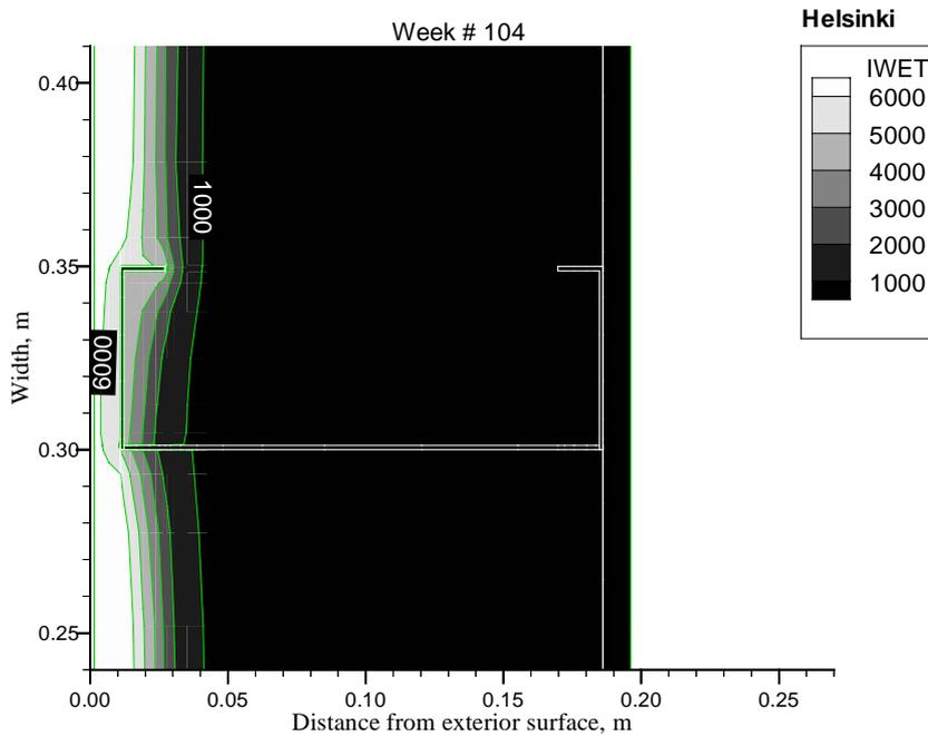
Figure 14. Contour plot of the accumulated time of wetness in the layers of the steel frame wall without exterior insulation. Exterior conditions: Helsinki weather data. Length of the simulated period is 2 years (104 weeks). Arrow shows the location of the highest contour value /14/.
