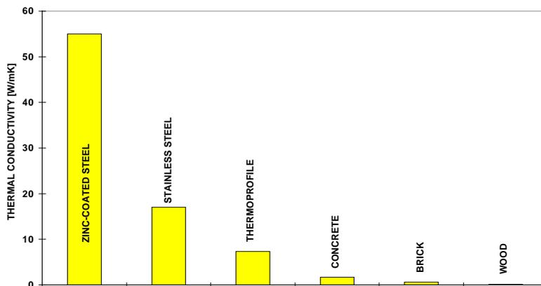
Figure 5. Thermal conductivity of various building materials used in load-bearing structures. Equivalent thermal conductivity for the thermopile.
