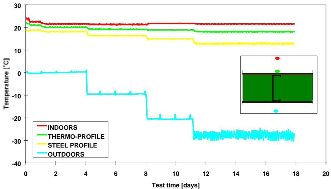
Figure 8. Surface temperatures of a light steel-framed wall according to a laboratory weather test.
