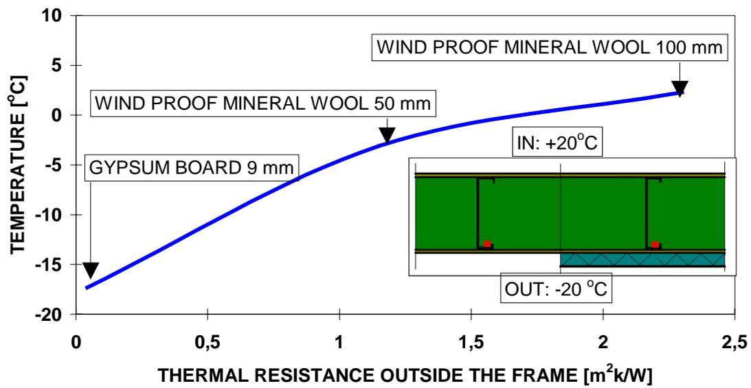
Figure 9. The effect of thermal properties of wind proofing (see Figure 1) on the temperature of outer parts of the frame /12/.
