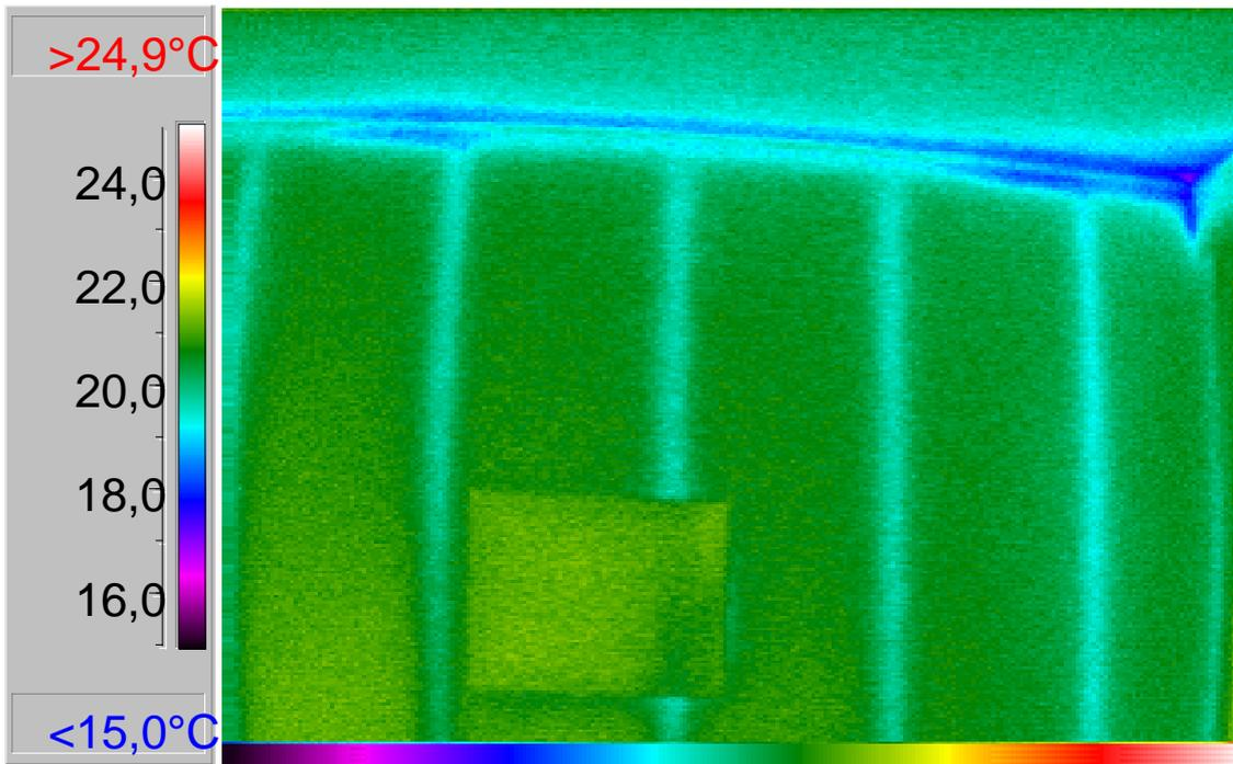
Figure 7. Infrared image of a steel wall.
