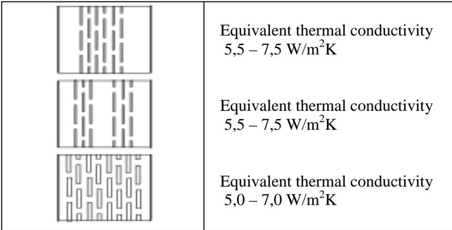
Figure 3. Perforation alternatives of a thermopile. Equivalent thermal conductivity takes into account the perforations filled with insulation material. Equivalent thermal conductivity depends on the properties of thermal insulation, the dimensions of the perforations and the dimensions of the solid steel between the perforations.
