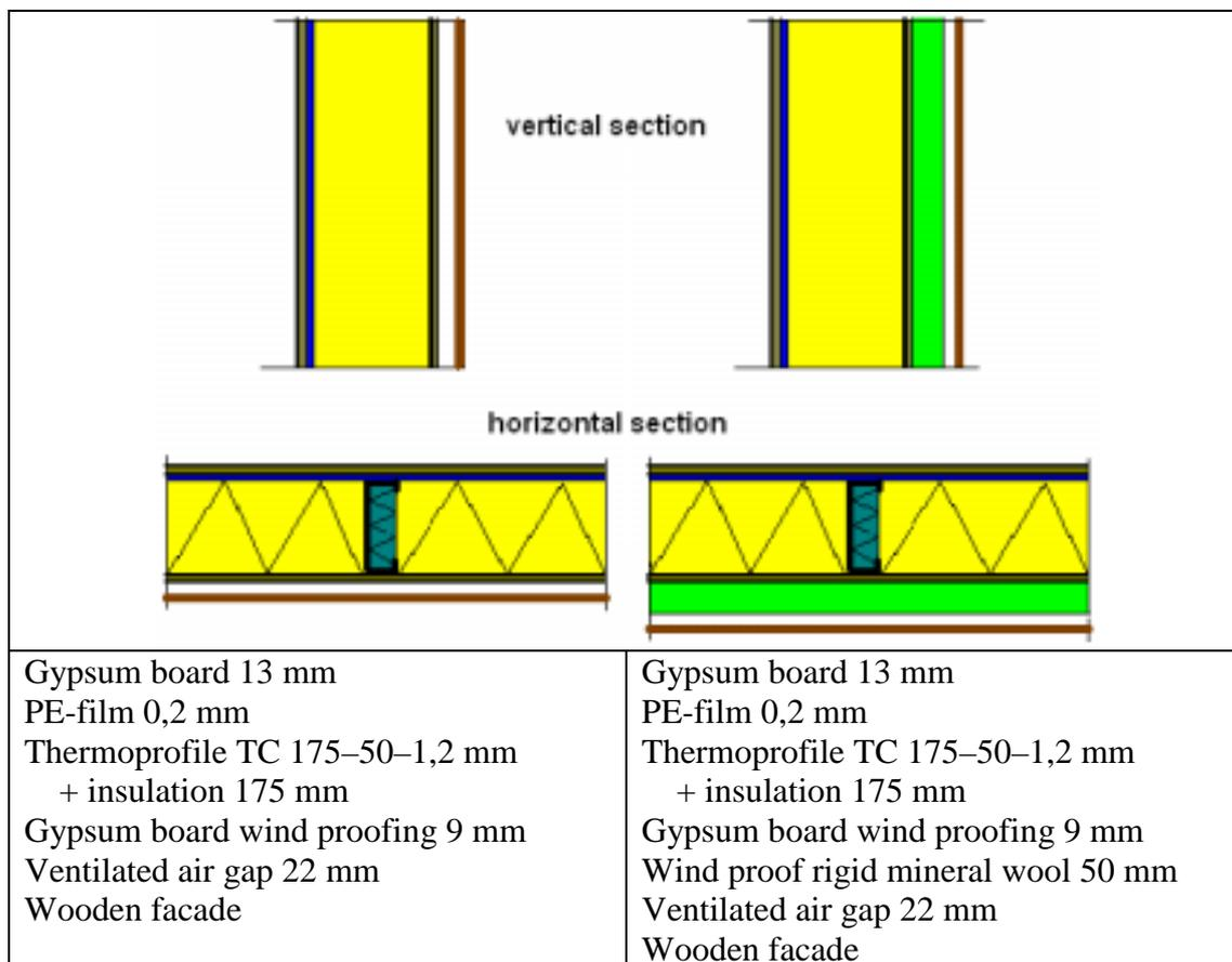
Figure 13. Illustration of the structure with perforated light gauge steel frame without and with exterior insulation.
