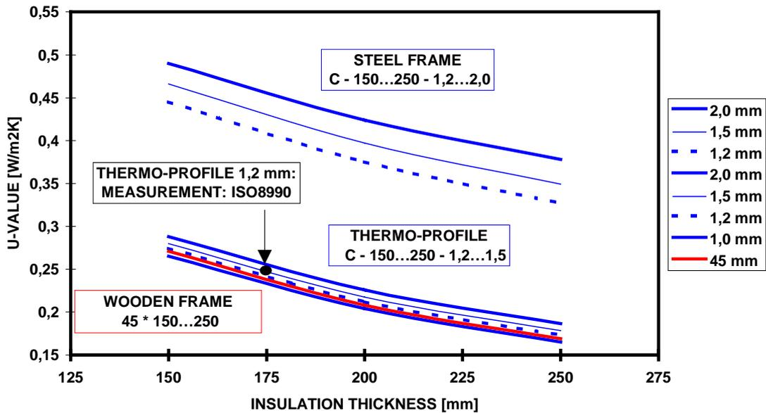
Figure 6. Calculated values of thermal transmittance for steel-framed and wood-framed walls /9/. The thermal benefit of the perforations in a steel member of a single frame structure is 40-50% depending on the insulation thickness of the wall.
