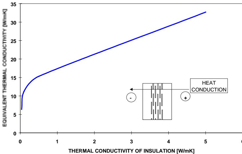
Figure 4. The effect of thermal insulation into the equivalent thermal conductivity of the typical Finnish thermopile /12/.
