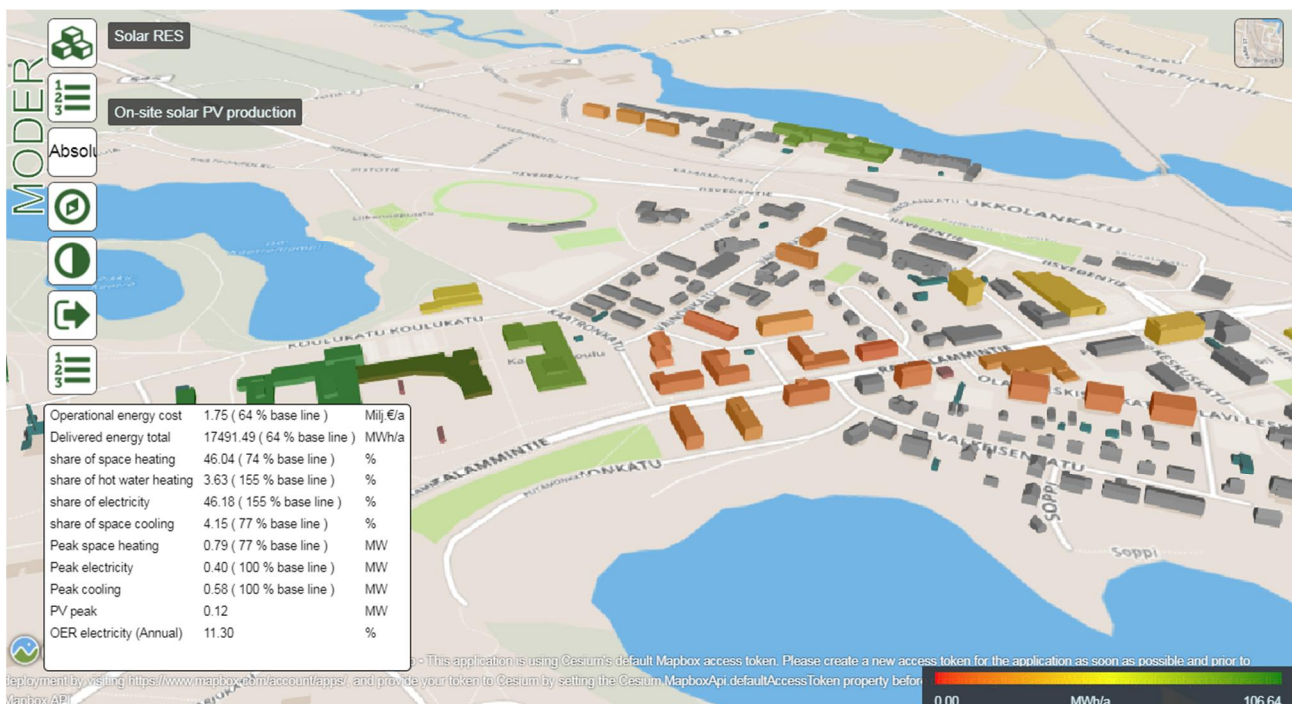
Figure 3 An example of the Step 2 scenario alternative on the solar electricity energy potential on the roofs of the selected buildings in the city of Suonenjoki centre in Finland. The KPI's and their relative change compared to the baseline are summarized in the left hand corner of the viewer.
