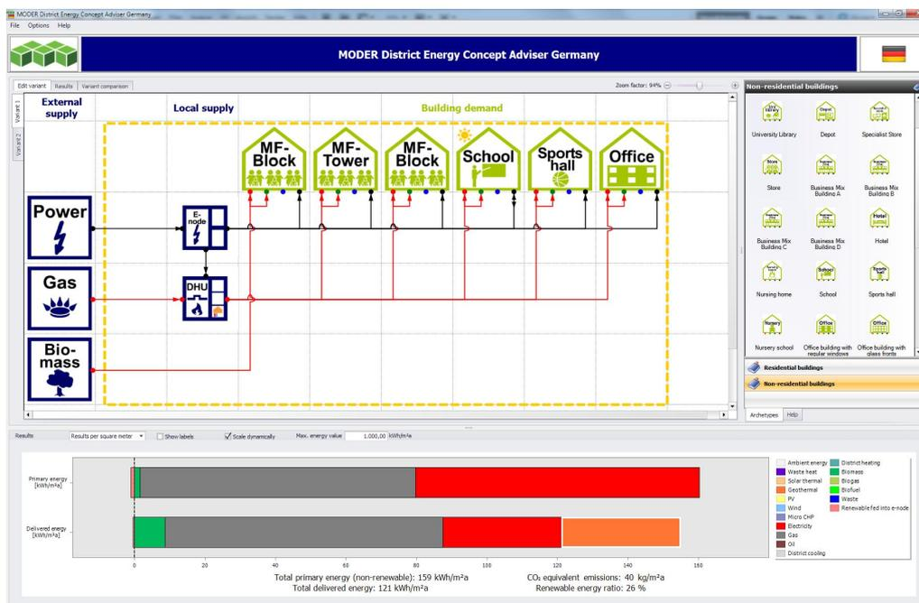
Figure 1: User-interface of the energy assessment of districts tool out of the D-ECA [7]
