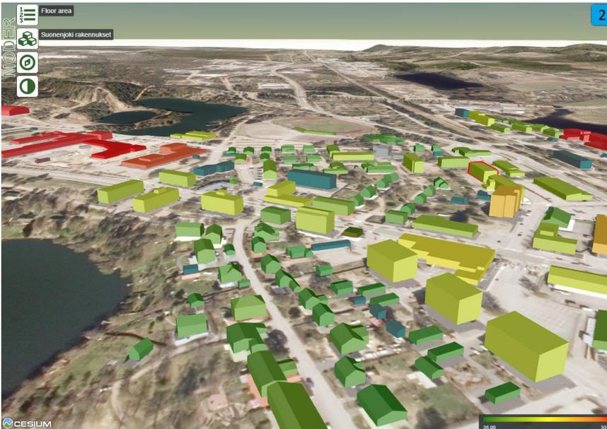
Figure 4: Test version of Apros simulation visualisation based on case Suonenjoki city information model. The colour code refers to improvements in energy performance of individual buildings [7]
