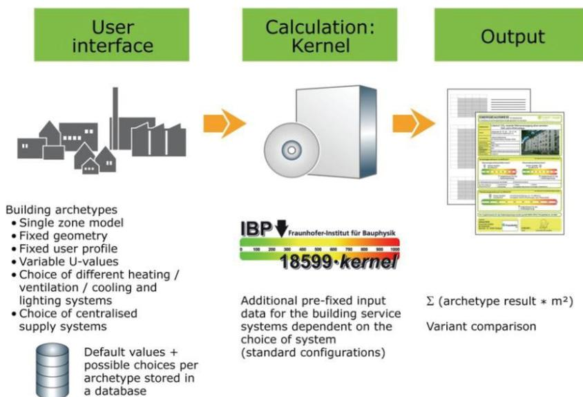
Figure 2: Software architecture of the tool energy performance assessment of districts as part [9]
